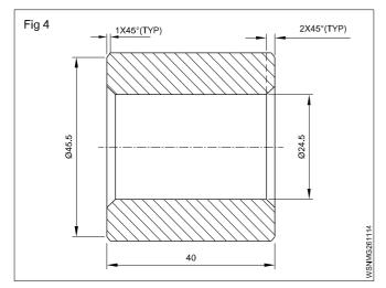
Component size =  $\emptyset 45.5 \times 40 \text{ mm}$ Raw material size =  $\emptyset 50 \times 45 \text{ mm}$ =  $\emptyset 5 \times 4.5 \text{ cm}$ Volume =  $\pi r^2 h$ =  $3.14 \times 2.5 \times 2.5 \times 4.5 \text{ cm}^3$ =  $88.313 \text{ cm}^3$ Weight = Volume x Density Density =  $7.8 \text{ gm/cm}^3$ Weight =  $88.313 \times 7.8 \text{ grams}$ = 688.841 grams= 0.689 KgCost of raw material = Rs.100/kgCost of material =  $0.689 \times \text{Rs.100}$ = Rs.68.90= Rs.68
