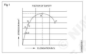
The ratio of ultimate stress to working stress (i.e. safe stress) is known as factor of safety. The ratio of ultimate load to the safe load may also be termed as factor of safety. It has no unit. Hence it is expressed in a number.
