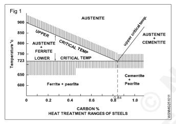
If the hot steel is cooled rapidly the austenite changes into a new structure called 'Martensite'. This structure is very fine grained, very hard and magnetic. It is extremely wearresistant and can cut other metals.
