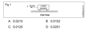
7 Calculate the pulling force required for the figure shown.
