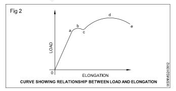
A metal (say mild steel) is subjected to increasing load and the extensions are measured with an extensometer. On plotting a graph between the loads and elongations produced, in the beginning, there is a straight-line relationship. It continues up to 'a' which is called the limit of proportionality, i.e. up to 'a' in Fig 2 'Stress is proportional to strain'.
